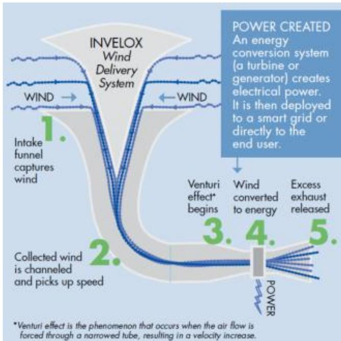
Figure 1 Schematic of the INVELOX wind delivery system showing its key parts
