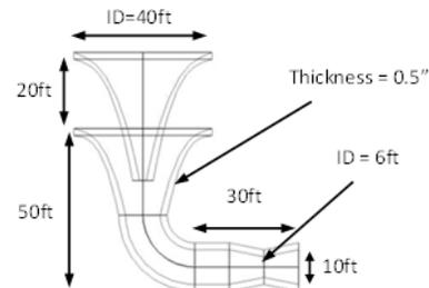
Figure 2 Detailed dimensions and geometry of omnidirectional INVELOX
