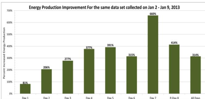
Figure 7 Daily energy production improvements - the INVELOX with respect to traditional turbine-tower systems
