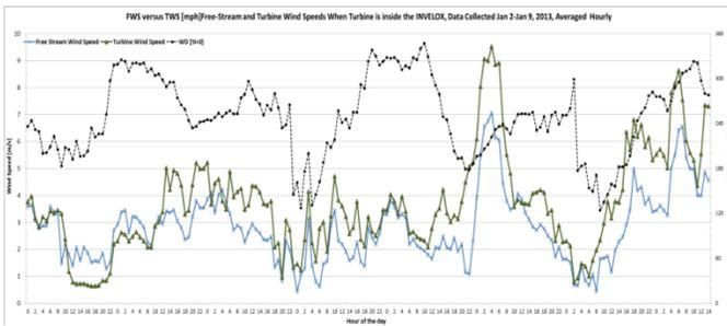
Figure 6 Free-stream and turbine wind speed and wind direction data measured over 8 days
