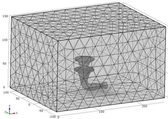
Figure 3 CFD model showing INVELOX and virtual wind tunnel
